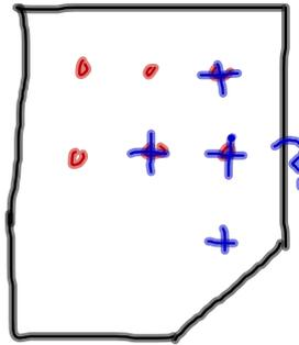
Can't implement Laplace molecule at a point next to the boundary if it's not a Dirichlet boundary.
