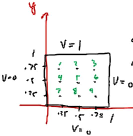
at node #1:  $1 + V_4 + 0 + V_2 - 4V_1 = 0$
