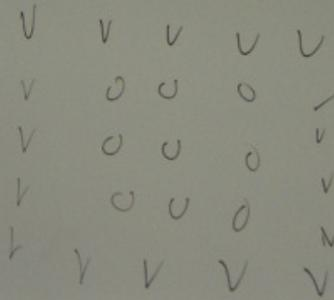
$$V_o^{new} = \frac{V_{\rightarrow}^{old} + V_{\leftarrow}^{old} + V_{\uparrow}^{old} + V_{\downarrow}^{old}}{4}$$
